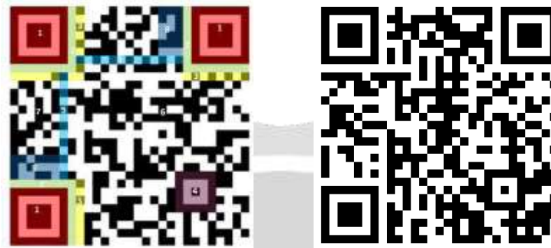
Fig -1: Schematic Diagram of QR Code
